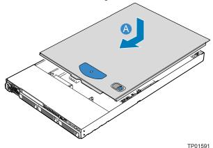
Figure 8. Installing the Chassis Cover
